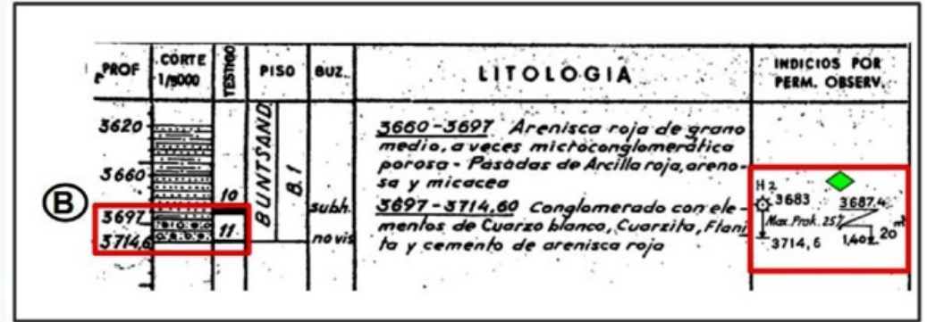
Hydrogen shows (100% of gas) from the composite log (ENPASA, 1963)
